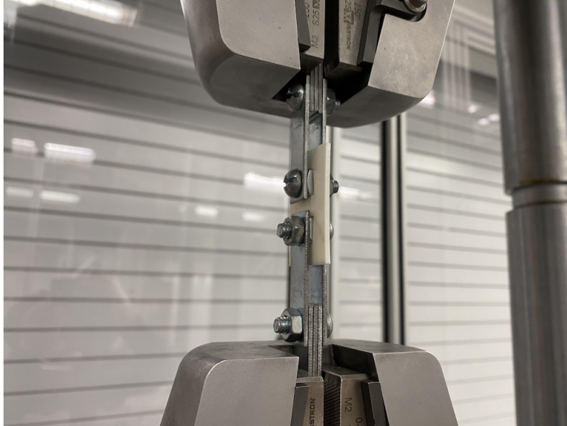
Figure 3.3: A 3D printed part being tested on a universal testing machine (Instron 600DX), with square nuts in the trapezoidal holes. The machine moves at a speed of 20 mm/min and stops when the object breaks or by a manual stop.
